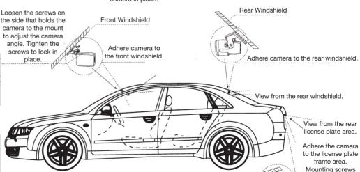
Loosen the screws on the side that hold the camera to the mount
