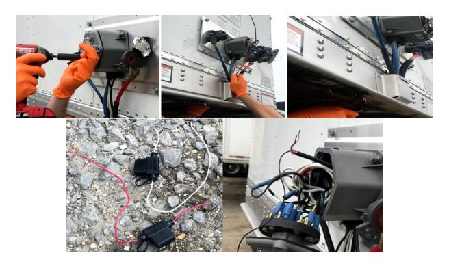
• After the Trailer Tracker Cable is run, splice the red & white wire from the Trailer Tracker unit into the trailers "Constant Power". Next, splice into the trailers "Ground" and connect the black wire from the trailer tracker harness. Please note to tap into the wire and not the connector as it becomes very tight in the plug section.
