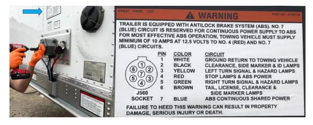
When installing the wire through the case you may need a small snake line as it is a tight access.
