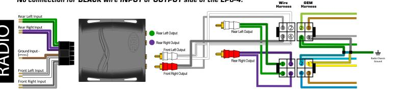
Ground Cable: If noise present try connecting to ground otherwise no connection
