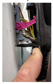
Run the camera wire thru the bottom portion of the boot as well as bottom cavity entering the cab of the truck. Purple clip must stay horizontal until clip is reinserted into connector
