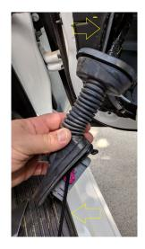
Pull the entire boot thru the speaker opening, run a zip tie or fish lead from one end to the other. Use this to pull camera wire thru
