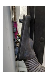
Reinstall the door boot cab side clip starting from the bottom and clipping back into place at the top
