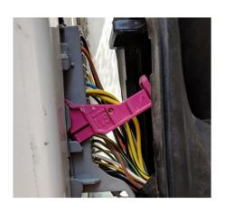
Use panel removal tool to unclip the purple connector and fold to a horizontal position
