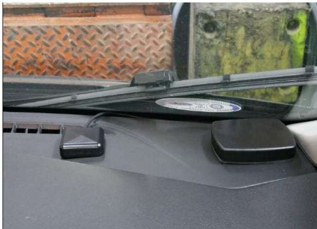
CRX GPS and LTE antenna properly installed on the Vehicle Dash DO NOT ATTACH THE LTE ANTENNA ONTO A METAL SURFACE
