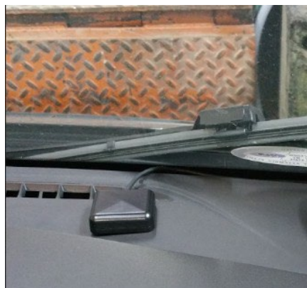
CP4 GPS antenna properly installed on the Vehicle Dash
